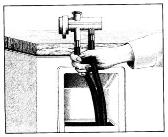
Press down on the thumb release. Lift the connector up onto the faucet and release your thumb pressure so the connector is held firmly in place.
